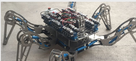
'Latro', an agile robotic spider, is one of the most recent additions to the array of tools available to deal with nuclear material in fuel ponds.
